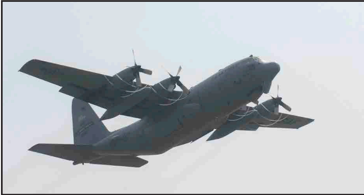
The C-130 is a rugged aircraft capable of transporting personnel and material within an operational theater. Though smaller, less expensive, aircraft are also effective in Africa, it is difficult to match the cargo capacity and short takeoff space of the C-130 (left)
