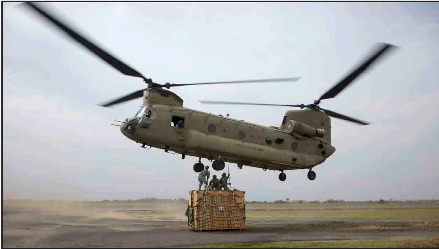
Riggers attach a sling load to a CH-47 Chinook helicopter during an airlift operation, Roberts International Airport, December 2014. The mission was to airlift incinerators to a new Ebola treatment facility built in support of Operation United Assistance
